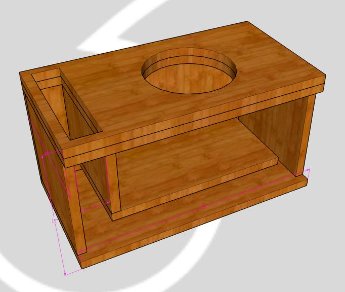
This is a 1.5 cube (42L) slot ported box tuned to 37Hz designed for good bandwidth and accuracy.
