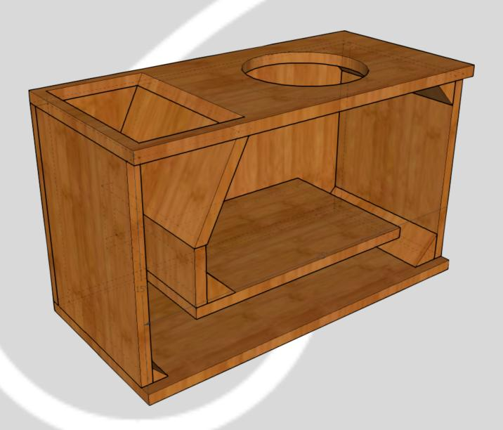
This is a 1.35 cube (38L) slot ported box tuned to 43Hz designed for good bandwidth and accuracy.
